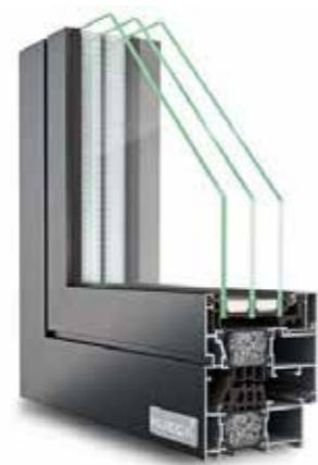
Lambda 77L/XL • thermally insulated, 77 mm profile depth
