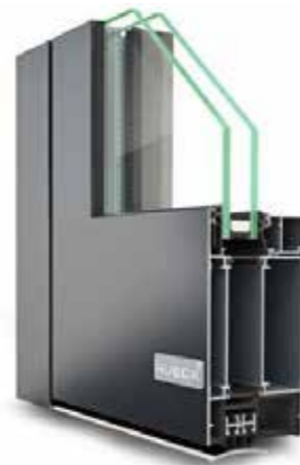
Lava 77-S • smoke protection doors, thermally insulated, 77 mm profile depth
